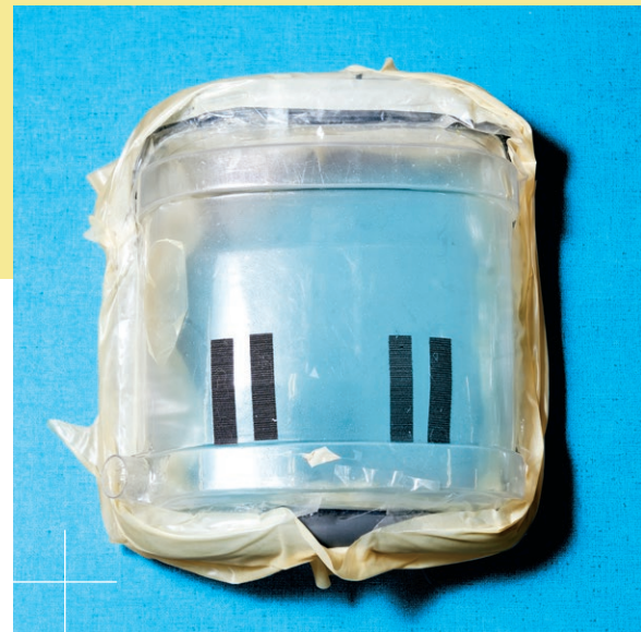
The shell of the first prototype of the Right Air vest mirrored the shape of existing commercial ventilators. Brenner and Swoboda used simple rubber sheeting to produce a seal between the vest and the wearer's body.
