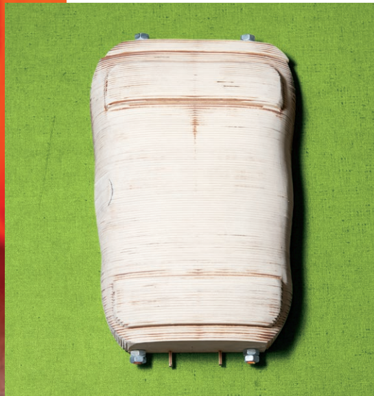
A shape form for molding a version of the plastic vest shell was laser cut in the NextFab woodshop of thin slices of wood.
