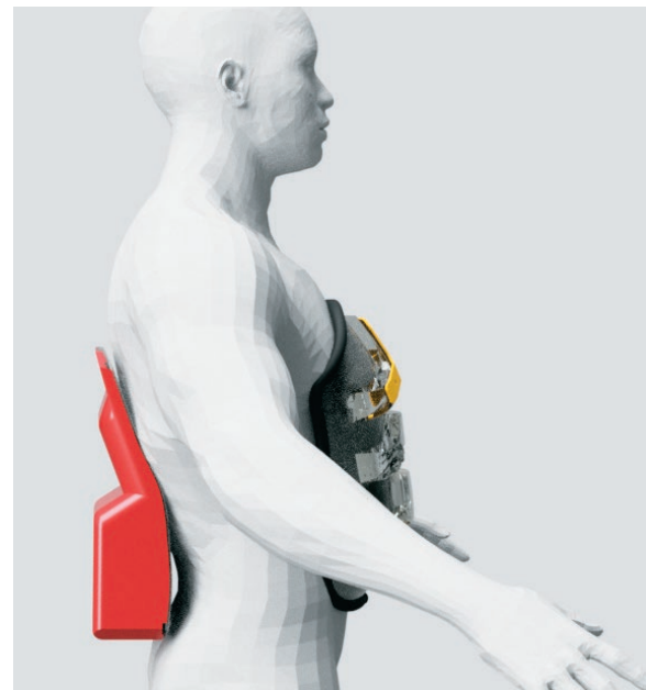
A pump worn on the back creates negative and positive air pressure inside of the shell to pull or push the patient's chest.
